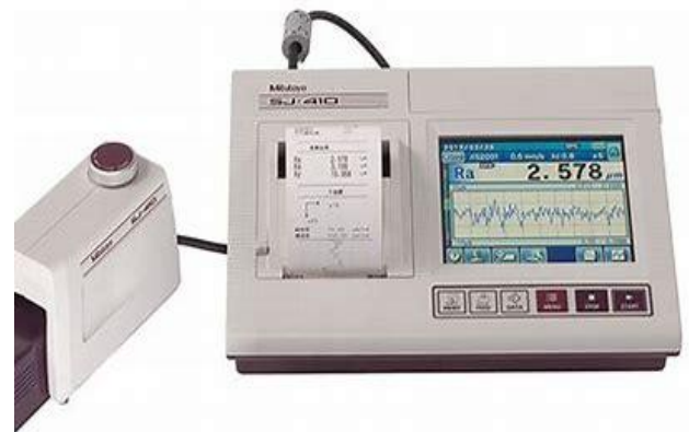
Fig. 2: MITUTOYO 178-602 Surface Roughness tester measuring the roughness of surface machined by milling machine
