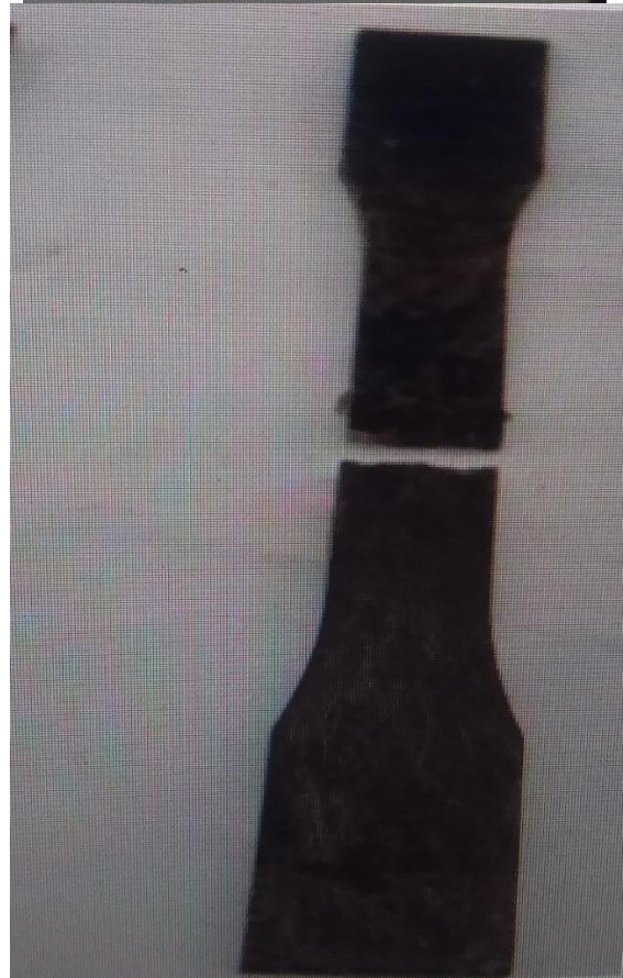
Fig. 3: Tensile specimen before and after testing
