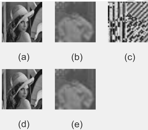
Fig. 1: (a) is original image, (b) original watermark image, (c) watermark image after chaos with optimized GA encryption, (d) is the watermark embedded image and (e) is the watermark image after extraction and decryption process.
